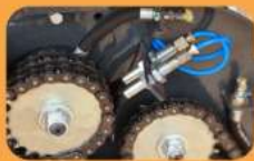
Automatic Centralised Lubrications System With Cleaning Brush
