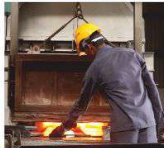
WALKING BEAM FURNACE
